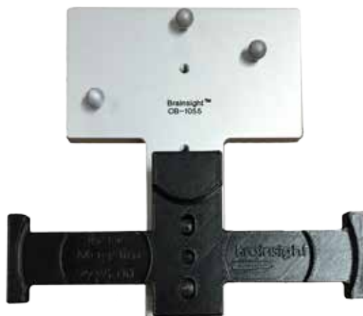
A: Calibration jig for a common coil (Magstim 9925 or Alpha coil) on the adapter.
